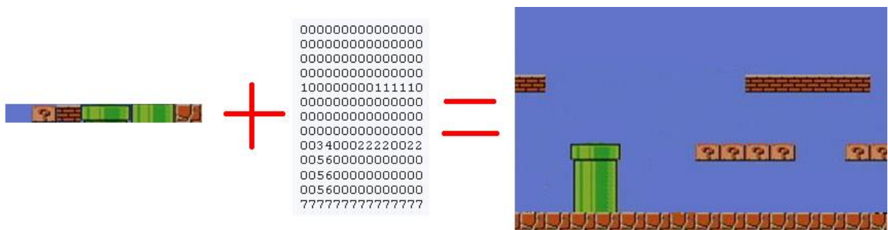
FIGURE I.8.4. – Schéma Tiles mapping
